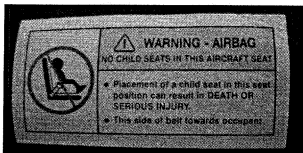
Representative Seatbelt Warning Label Note: Label side of belt goes towards occupant.
